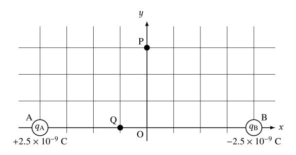
(1) Which is the correct direction of the resultant electric field at P = (0, 3.0 m)? Choose the correct answer from (a) – (h) in the following figure and write the letter of your choice.
